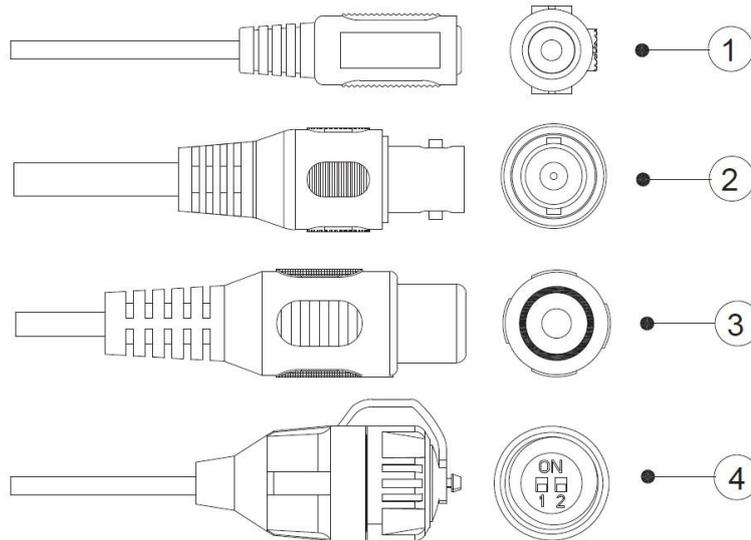
For more information about cable ports, see Table 2-1; for the operation method of ④ (DIP switch), see Table 2-2.
